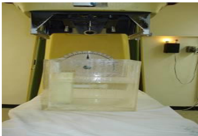
Figure 4: Calibration set up under the tele Cobalt unit in multi tube method therapy.
